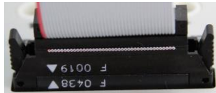
Fig 3: Correct orientation while plugging flat-ribbon-cables
