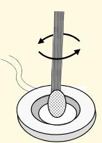
Through the large opening of ring-shaped electrodes abrasion can be performed by means of a cotton swab.
