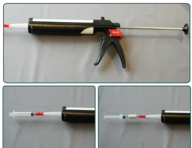
Fig. 3: By using a skeleton gun and the special adaptor, the gel can be filled bubble-free into the syringe. The adaptor fits syringes with or without thread.
